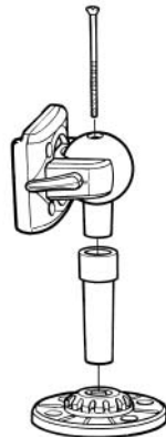
Figure 9. Install the mount to a flat surface using either the adhesive pad or screw mount.
